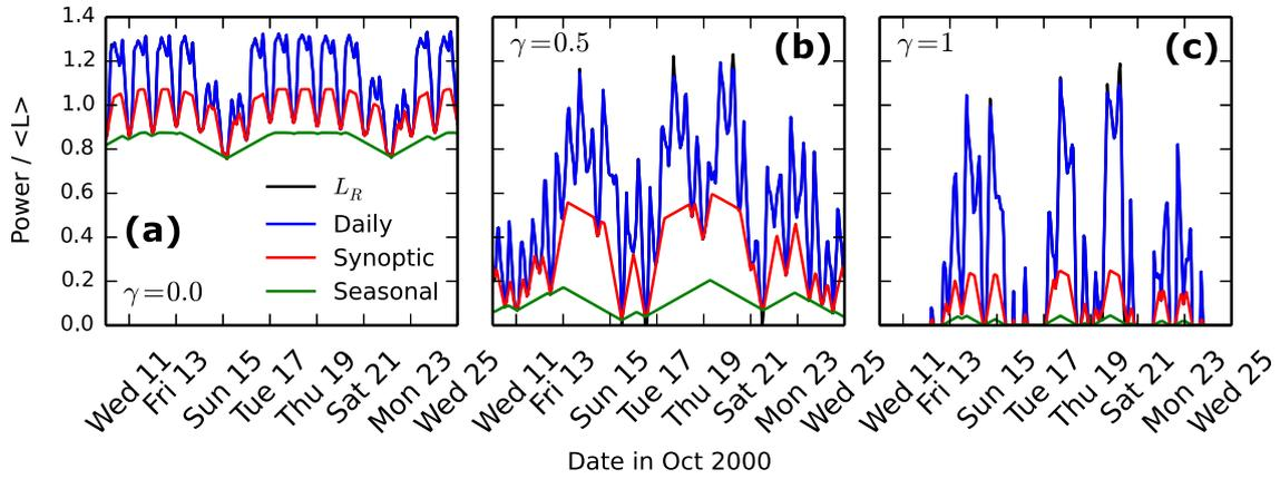
**Fig. 3.** A two-week period of the modelled dispatches for Germany for  $\gamma = 0, 0.5, 1$  in panels (a,b,c), respectively. The dispatches of the slow, medium, and fast flexibility classes (green, red, blue lines) are plotted cumulatively, and together match the (residual) load (black lines, mostly overlapped by the blue lines) at almost all times. (For interpretation of the references to colour in this figure legend, the reader is referred to the web version of this article.)
