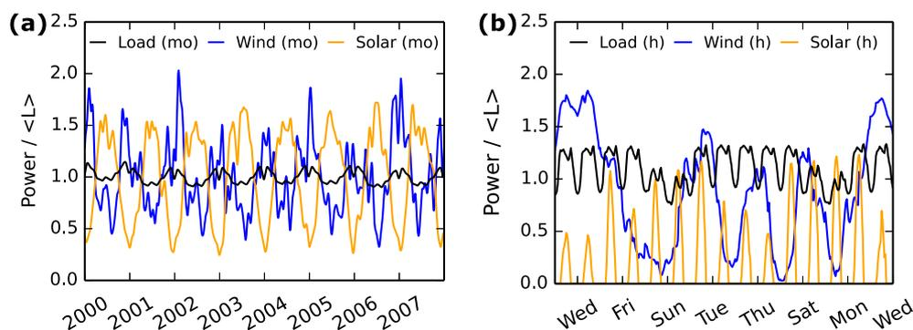
**Fig. 1.** Examples of time series of load and weather-based wind/solar generation in Germany based on data described by Heide et al. [1]. (a) All eight years of data, smoothed over one month to see long-term trends. (b) Hourly load and generation for two example weeks in October 2000. All time series have been normalized to an average load of one.
