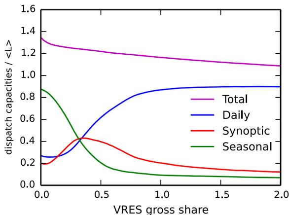
**Fig. 2.** Modelled optimal backup capacities in units of the mean load versus VRES gross share  $\gamma$  for Germany. The blue, red, and green lines correspond to the fast, medium, and slow flexibility classes, respectively. The sum of the three capacities is given by the magenta line. (For interpretation of the references to colour in this figure legend, the reader is referred to the web version of this article.)
