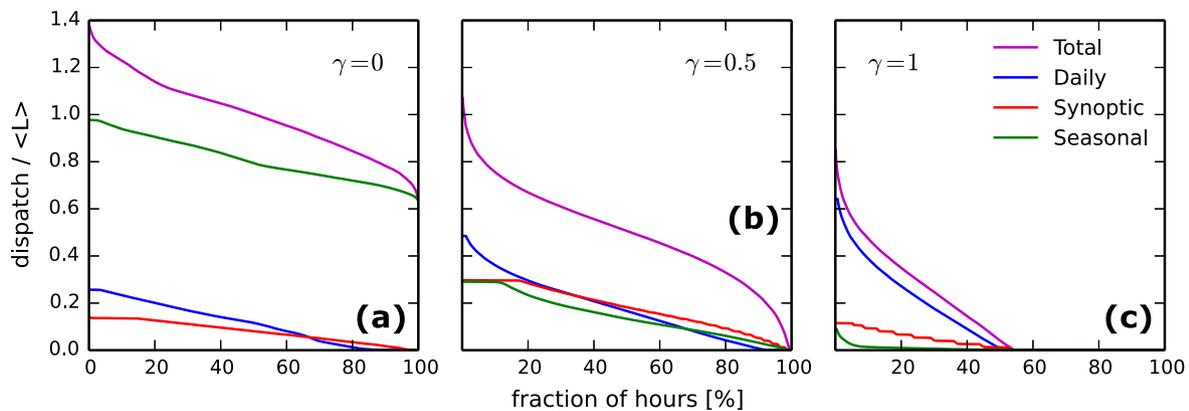
**Fig. 6.** Dispatch duration curves for the three flexibility classes and their sum at  $\gamma = 0, 0.5, 1.0$  (a,b,c), which show the hourly dispatch not in chronological, but in decreasing order against quantiles of hours. Here 100% of the hours correspond to the 8 years of data.
