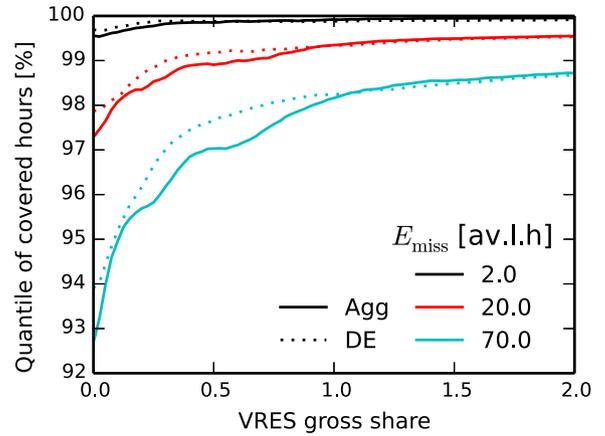
**Fig. A.10.** Quantiles of the number of covered hours at  $E_{miss} = 2, 20, 70$  av.l.h. in eight years (black, red, cyan) as a function of VRES gross share  $\gamma$  for aggregated Europe (solid) and isolated Germany (dotted). (For interpretation of the references to colour in this figure legend, the reader is referred to the web version of this article.)
