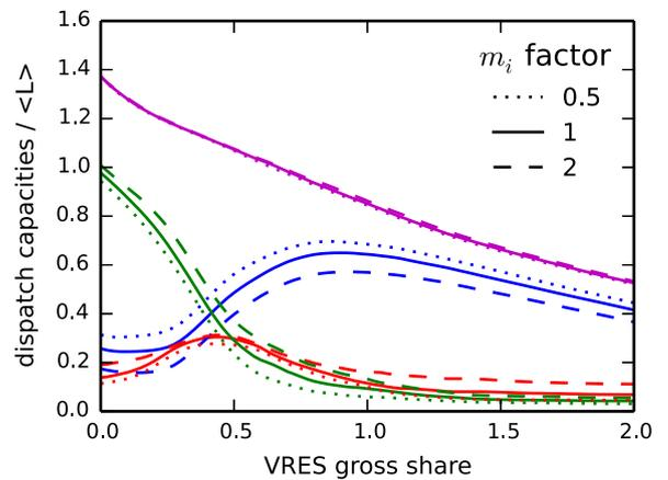
**Fig. 8.** Modelled capacities assuming half (dotted) and twice (dashed) the reference (solid) ramp rates ( $m_i$  remain unconstrained), respectively, versus  $\gamma$  for aggregated Europe. Total fast, medium, slow capacities are shown as magenta, blue, red, green lines. Solid lines are the same as in Fig. 4. (For interpretation of the references to colour in this figure legend, the reader is referred to the web version of this article.)
