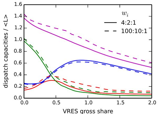
**Fig. A.11.** Modelled capacities assuming relative ratios of the capacity weights  $w_f : w_m : w_s = 4 : 2 : 1$  (solid, reference model) and  $100 : 10 : 1$  (dashed) versus  $\gamma$  for aggregated Europe. Total, fast, medium, slow capacities are shown as magenta, blue, red, green lines. Solid lines are the same as in Fig. 4. (For interpretation of the references to colour in this figure legend, the reader is referred to the web version of this article.)
