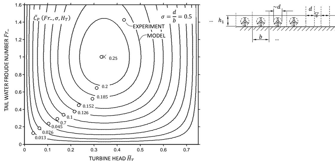
**Figure 1:** Coefficient of performance for a tidal turbine fence
